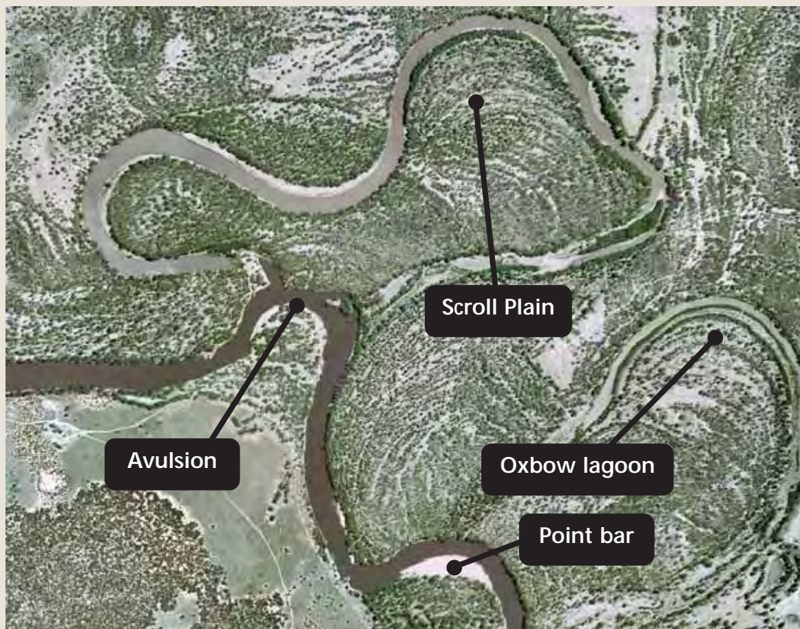
Figure 3.1 Air photo showing meander channel features of the River Murray floodplain, Retail Bend and Murray-Kulkynne Park (see Figure 3.2 for location).
