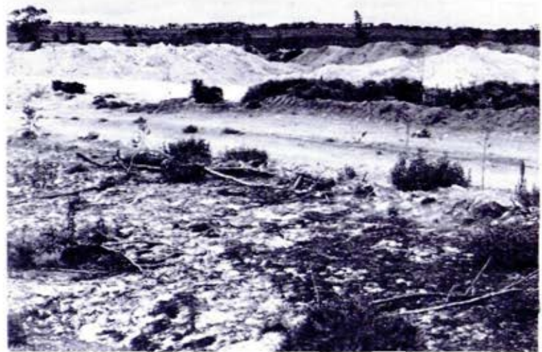
Extraction of powdered gypsum from a dune at Bailey's Plains
